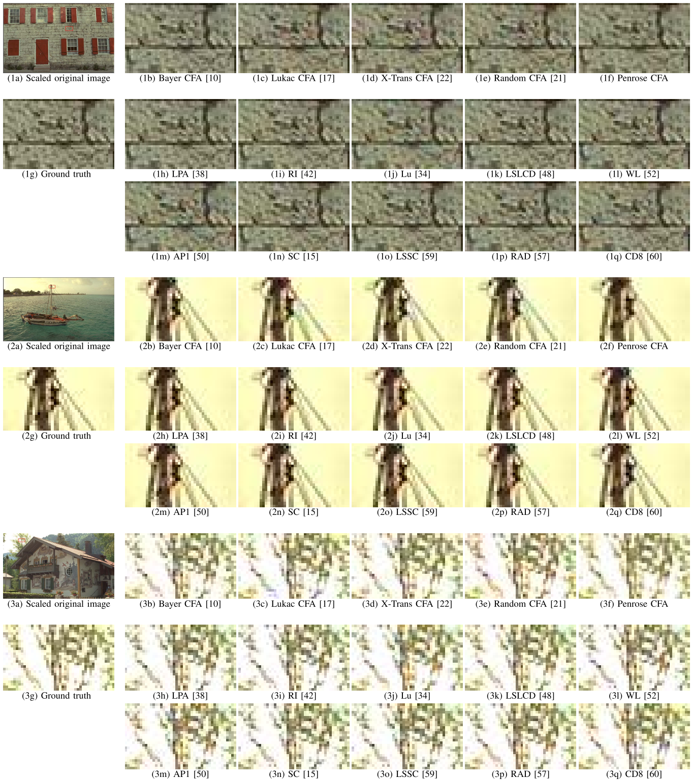
Fig. 7. More blowups of demosaicked images in the Kodak dataset. From top to bottom, the images are from #1, #6, and #24 Images of the Kodak dataset, respectively. In each group, (a) is the scaled original image, in which the red rectangle indicates the selected patch to blow up; (b)-(e) and (f) are the images demosaicked from raw images by regular RGB CFAs and Penrose CFA, respectively; (g) is the ground truth; (h)-(q) are the images demosaicked by the state-of-the-art demosaicking methods on the Bayer CFA [10]. We can observe that the Penrose demosaicked images are almost perfect, while all other images have false color.
