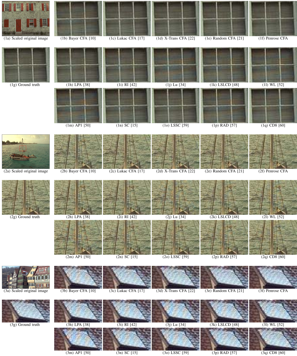
Fig. 6. Blowups of some demosaicked images in the Kodak dataset. From top to bottom, the images are from #1, #6, and #8 Images of the Kodak dataset, respectively. In each group, (a) is the scaled original image, in which the red rectangle indicates the selected patch to blow up; (b)-(e) and (f) are the images demosaicked from raw images by regular RGB CFAs and Penrose CFA, respectively; (g) is the ground truth; (h)-(q) are the images demosaicked by the state-of-the-art demosaicking methods on the Bayer CFA [10]. From all the three groups of images, we can clearly see that the images demosaicked from raw images by Bayer CFA [10], Lukac CFA [17], and X-Trans CFA [22] have severe false color artifacts at the window (false blue and yellow color artifacts), around the mast (false blue and yellow color artifacts), and on the roof of skylight (color stripe in the snow-covered area), while those by Random CFA [21] and Penrose CFA have better subjective quality.
